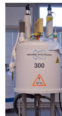
NMR 300 MHz equipped with QNP probe and ^{19}\text{F} selective probe
